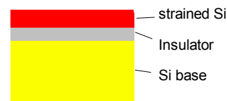
Figure 3. In sSOI, the strained Si is bonded directly to the insulating layer.
